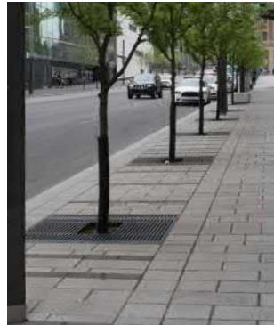
✓ Tree grilles aligning with paving and utilising below-ground wires and guys
