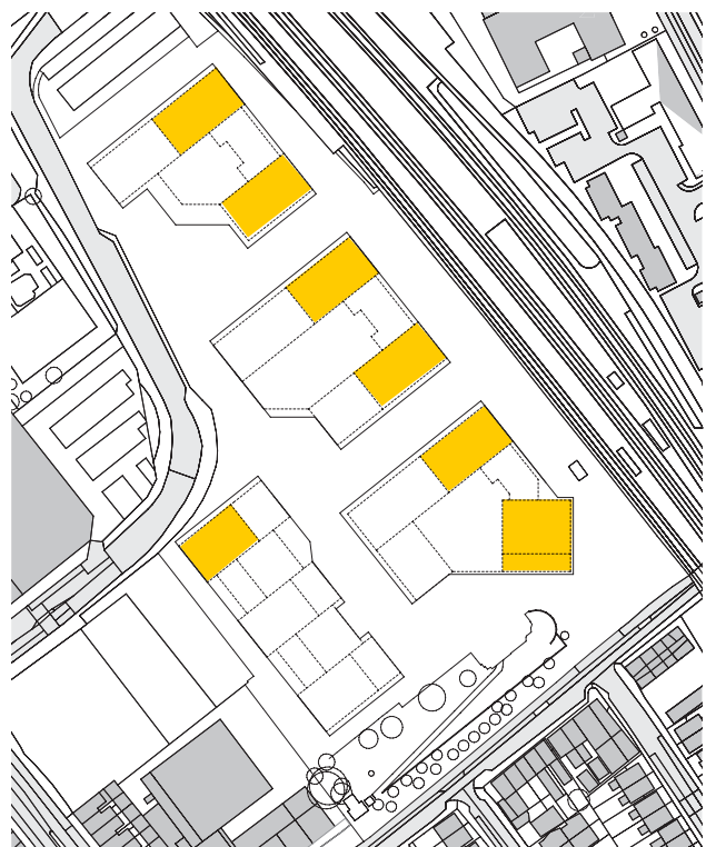
Above - Figure 11. Diagram indicates areas of maximum heights within each development plot
