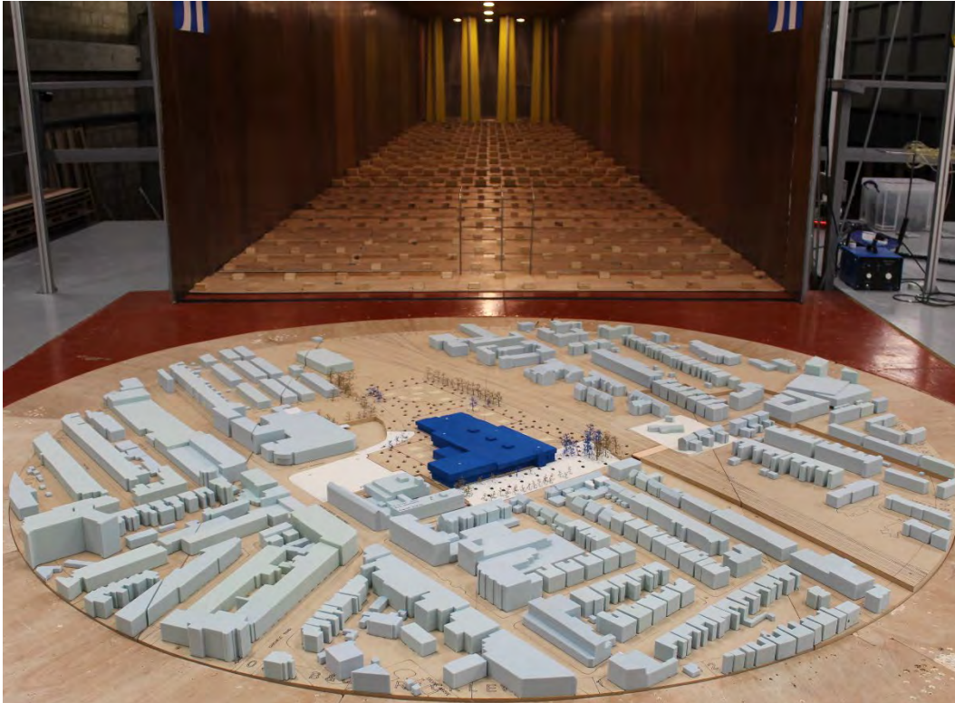
Figure 16: Existing Site with Existing Surrounding Buildings (Configuration 1) - View in the Wind Tunnel (from the south)
