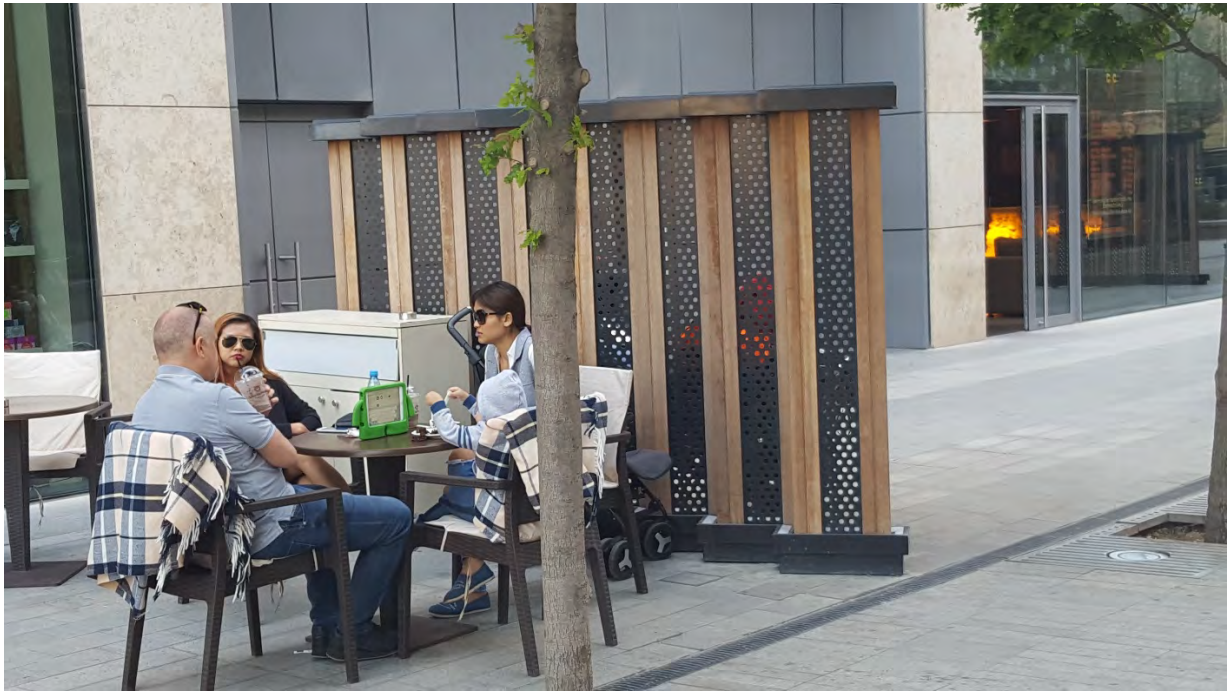
Figure 27: Porous Screen to Mitigate Wind Conditions for Seating Areas
