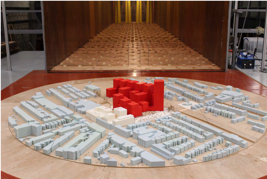
Figure 20: Proposed Development with Cumulative Surrounding Buildings and Existing Landscaping (Configuration 3) – View in the Wind Tunnel (from the south)
