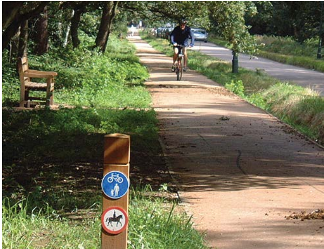
Flexibility in sign use: small version of the shared-use path sign as part of context-sensitive design
