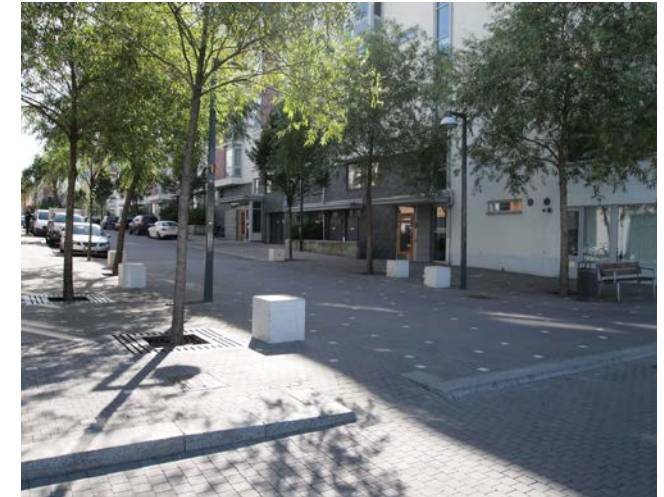
Continuous footway treatments in Stockholm. Note the dropped kerb to allow level access by cycle
