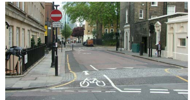
No entry with 'except cycles' plates, and raised table entry
