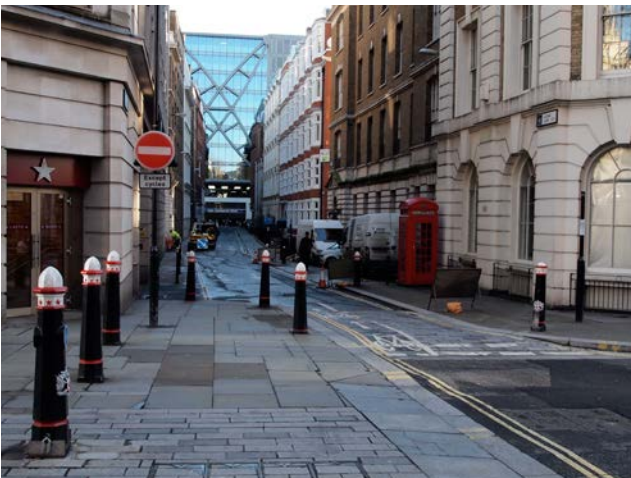
Typical entry treatments in the City of London, with visual contrast with carriageway: at a narrow street with cycle contraflow (Cloak Lane, left) and at a two-way street (Trump Street, right)
