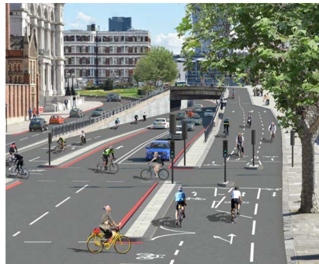
Visualisation, showing cycle movements separated at signalled junction
