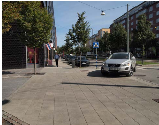
Continuous footway treatments in Stockholm. Note the dropped kerb to allow level access by cycle
