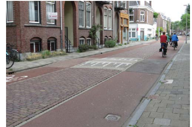
Example from Utrecht: (left) cycle street with mixed traffic, (right) cycle street with cyclists at the side.
