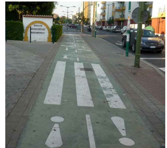
Pedestrian crossing over a cycle track in Seville, with extra warning for cyclists
