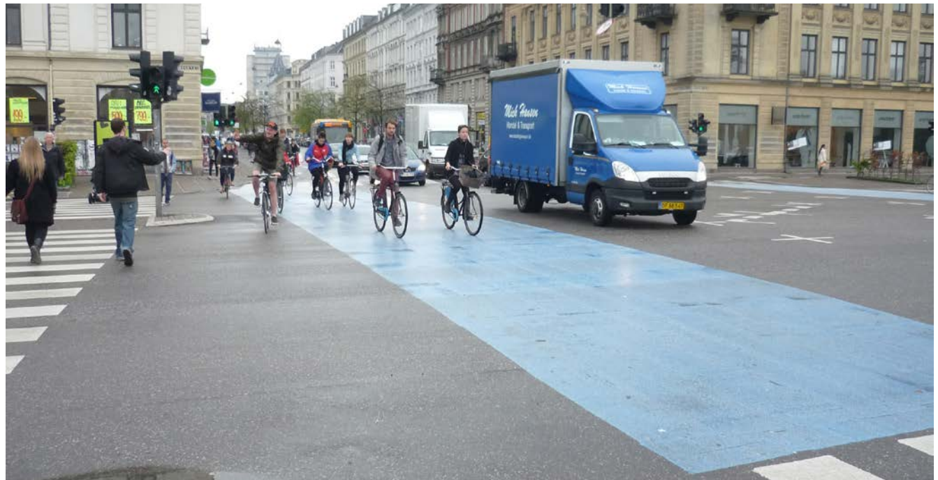
Use of coloured surfacing for cycling through junctions in Copenhagen
