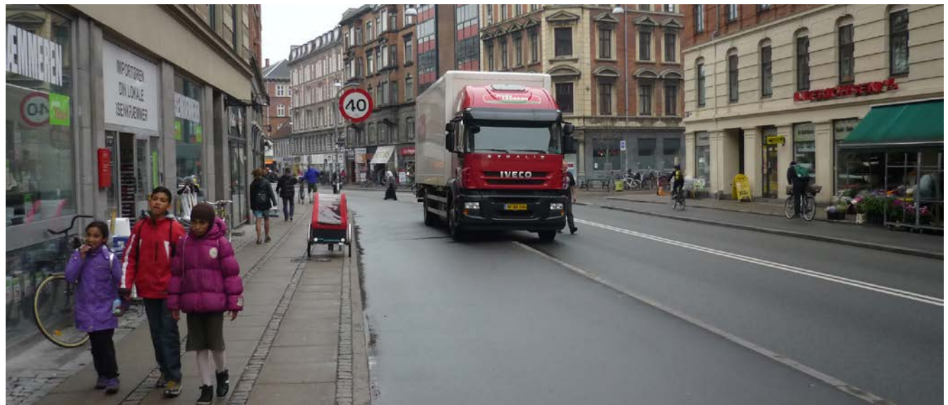
Loading across stepped tracks with low step up from the carriageway – Utrecht (top), Copenhagen (bottom)
