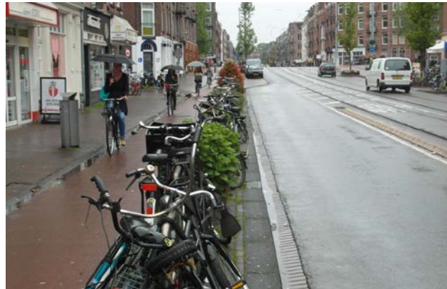
Segregating strip used for cycle parking, Utrecht
