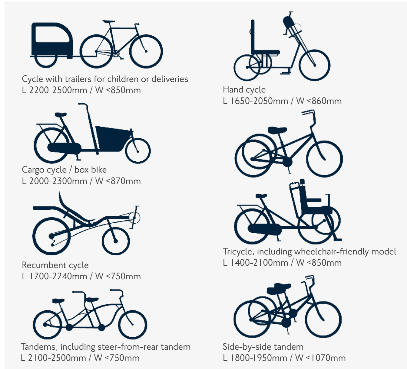
Figure 3.4 Indicative dimensions of typical ‘non-standard’ cycles
