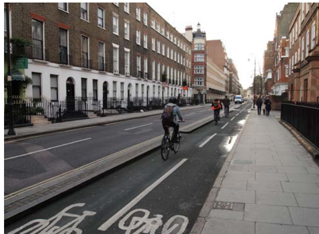
Two-way and contraflow segregated lanes/tracks: Tavistock Street (left) and Bury Place (right)
