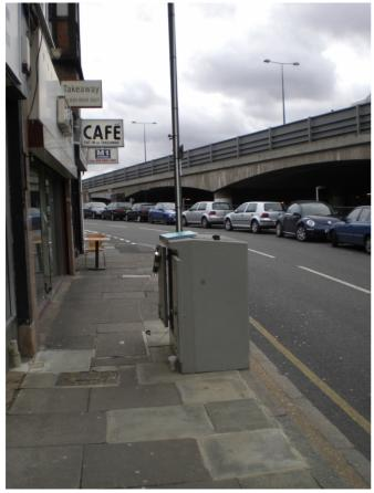
The monitor was located to represent relevant exposure which in this case is residential properties above the parade of shops. The bus station is to the right of the picture, underneath the elevated section of road (M1 motorway).
