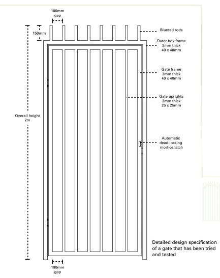
it should be removable so that any bulky items can be taken down the alley. Fixing for the top section should be accessible only when the gate is open. The side parts of the frame should be fixed to the wall (or post) through the frame using heavy duty fixings. These fixings should only be accessible when the gate is open.
